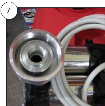
7 • Insert coupling (400LP-C2) into inlet of pump ensuring the coupling is fed through the captured nut 400LP-N first.
