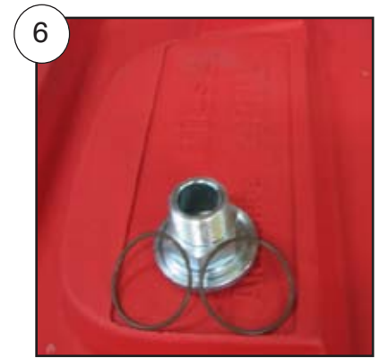
6 • Insert Viton O rings (BS136) to grooves on both sides of coupling (400LP-C2)
