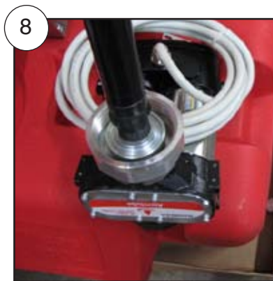
8 • Screw downtube into coupling
